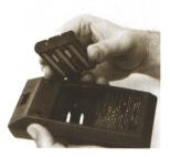
5. Insert the new battery pack so that its contacts face the calculator and contact is made with the battery connectors.
