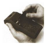
6. Insert the top of the battery door behind the retaining groove and close the door.
