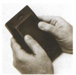
7. Secure the battery door by pressing it gently while sliding the two battery door latches upward.
