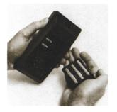
See if the battery connector springs have been inadvertently flattened inward. If so, bend them out and try the battery again.
